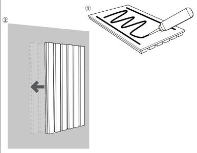
Note:Most adhesives will grab instantly,but take hours to adhere fully, so we Recommend putting 1-4 screws or finishing nails through the felt to hold the panels in place while theybond. The screws or nails can be removed from the felt once the adhesive has bonded to your wal
