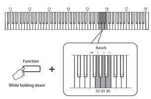
Press and hold the [Function] button, then press the [F5] key on the keyboard to turn off the Reverb.
