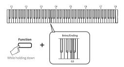
When the rhythm is playing back, press and hold the [Function] button, then press the [G3] key on the keyboard to end the rhythm, the Main Section will switch to the Ending.
