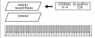
2 Press and hold the [Function] button, then press the [G6] key on the keyboard to turn on the Dual mode.
