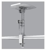
3.Loosen the knob 3, dial-in the perfect tilt angle to focus your tweeters to ear level. The speaker tilt angle is from 0 to 20 degrees. Tighten up the knob 3 after adjustment.
